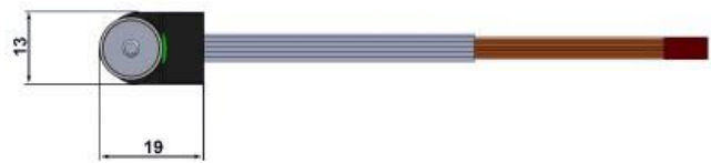
Schematic drawing of ROMO with factory installed encoder and custom leadscrew shaft. Dimensions (mm)
