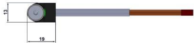
Schematic drawing of ROMO with factory installed encoder) and custom leadscrew shaft. Dimensions (mm)
